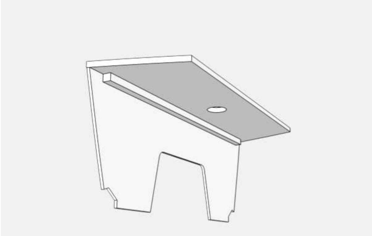
The partner sits on top of the frame. Edges are flush. The two parts are epoxy glued with a corner cleat. The section of the cleat is unimportant: 1" square is fine or use leftover plywood as for the trunk. Note that the cleat does extend all the way to the sides. Pay attention to squareness when gluing the parts, the frame must be perpendicular to the partner.
